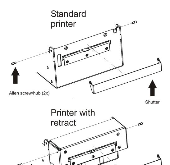
The shutter kit contains a shutter and two hub-screws. In addition to this, you need an 1.5 mm Allen-key.
